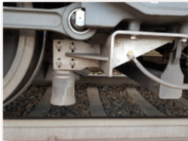
CORRail installed on a DB BR401 and optimally positioned close to the wheel
